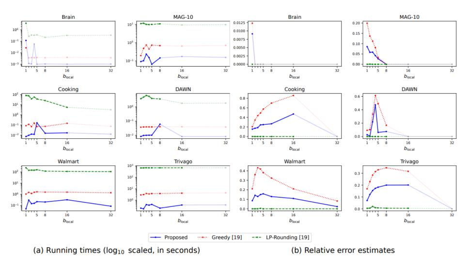
Figure 1: (a) Running times (in seconds, log scale) and (b) relative error estimates of the LOCAL ECC algorithms. Empty square markers denote trivial instances.
